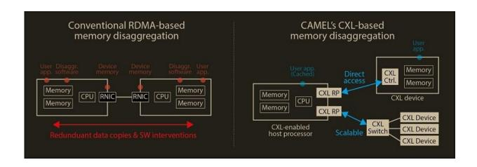
Figure 1. a comparison of the architecture between CAMEL's CXL solution and conventional RDMA-based memory disaggregation. Credit: KAIST
