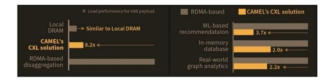
Figure 2. A performance comparison between CAMEL's CXL solution and prior RDMA-based disaggregation. Credit: KAIST
