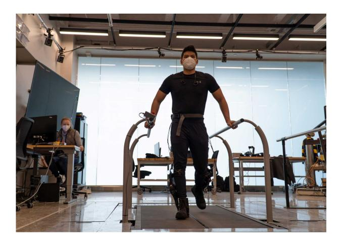
Leo Medrano, a PhD student in the Neurobionics Lab at the University of Michigan, tests out an ankle exoskeleton on a two-track treadmill. By allowing the user to directly manipulate the exoskeleton's settings while testing it on a treadmill, preferences that are difficult to detect or measure, such as comfort, could be accounted for by the users themselves. Credit: University of Michigan Robotics Institute
