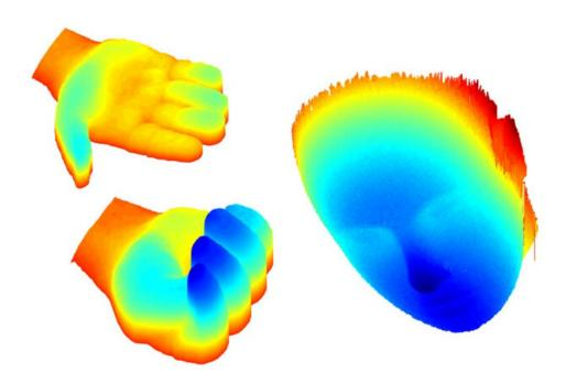
Duke researchers have shown that a new approach to LiDAR can be sensitive enough to capture millimeter-scale features such as those on a human face. Credit: Ruobing Qian, Duke University
