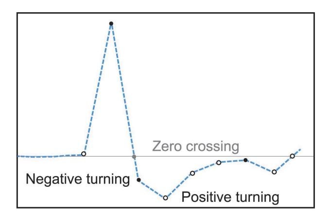
Supervised machine learning found that negative turning (black points) and positive turning (white points) amplitude measurements across a neutral zero line (grey points) happened in concert with rock fracture moments. Credit: Rui Liu, Texas A&M Engineering
