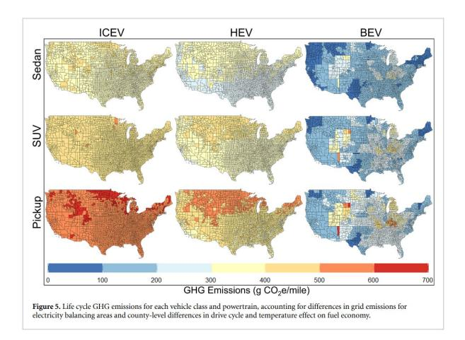
Life cycle greenhouse gas emissions for each vehicle class and powertrain. Average lifetime emissions account for differences in grid emissions for electricity balancing areas and county-level differences in drive cycle and temperature effect on fuel economy. Credit: From Woody et al. in
