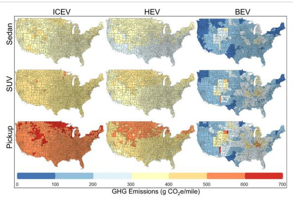
**Figure 5.** Life cycle GHG emissions for each vehicle class and powertrain, accounting for differences in grid emissions for electricity balancing areas and county-level differences in drive cycle and temperature effect on fuel economy.
