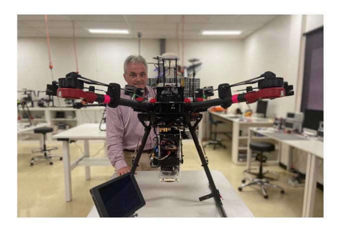
UniSA Professor Anthony Finn pictured with A DJI Matrice 600 drone with a payload capable of emitting or receiving acoustic signals. Credit: University of South Australia
