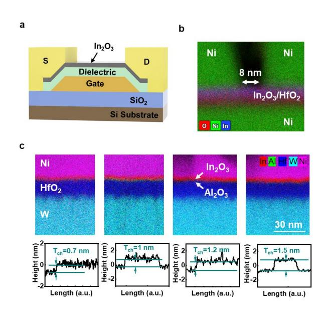
The ultimately scaled  $In_2O_3$  transistor with channel length of 8 nm and  $In_2O_3$
