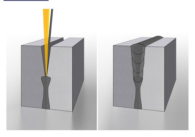
The laser beam is positioned at the joint between the two sheet edges to be welded, and a filler metal is inserted in front of it at the same time. The process results in a high-quality welded seam. Credit: Fraunhofer-Gesellschaft
