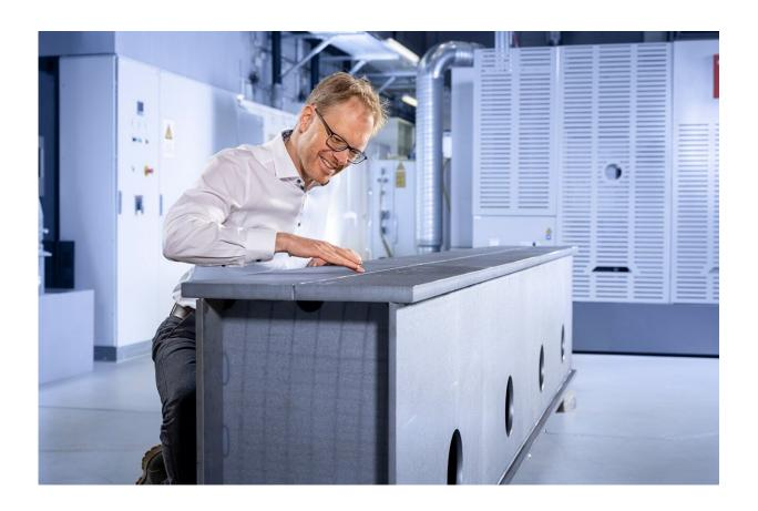
Researchers at the Fraunhofer IWS used an indoor crane segment made of S355J2 structural steel (4 by 0.75 by 0.5 meters) to demonstrate that the laser MPNG welding process they had developed reduces energy costs by up to 80 percent and filler material consumption by up to 85 percent compared to conventional welding processes. Credit: Fraunhofer-Gesellschaft
