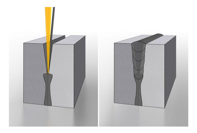
The laser beam is positioned at the joint between the two sheet edges to be welded, and a filler metal is inserted in front of it at the same time. The process results in a high-quality welded seam. Credit: Fraunhofer-Gesellschaft
