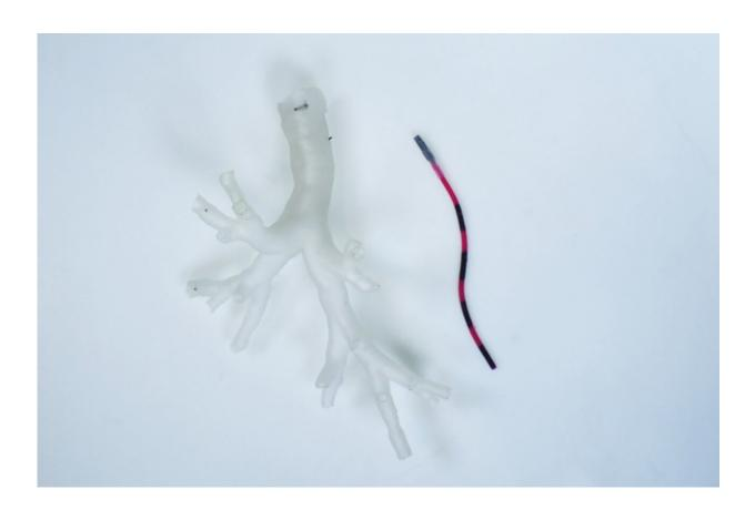
A life-size model of part of a bronchial tree built from anatomical data. A section of the magnetic tentacle robot is seen on the right. Image courtesy: University of Leeds. Credit: University of Leeds
