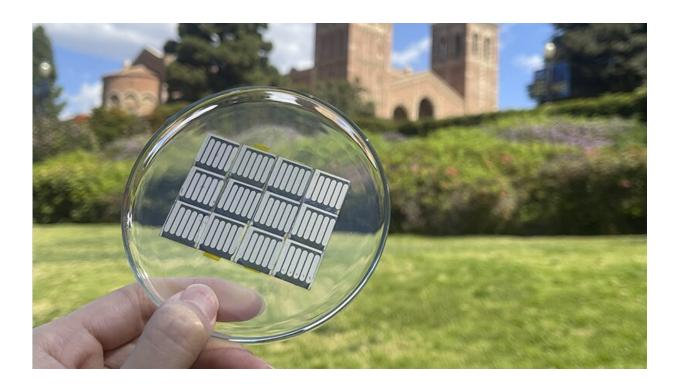
Photo of a thin film perovskite solar cell produced with a manufacturing process fix developed by UCLA researchers and colleagues. Credit: Shaun Tan/UCLA
