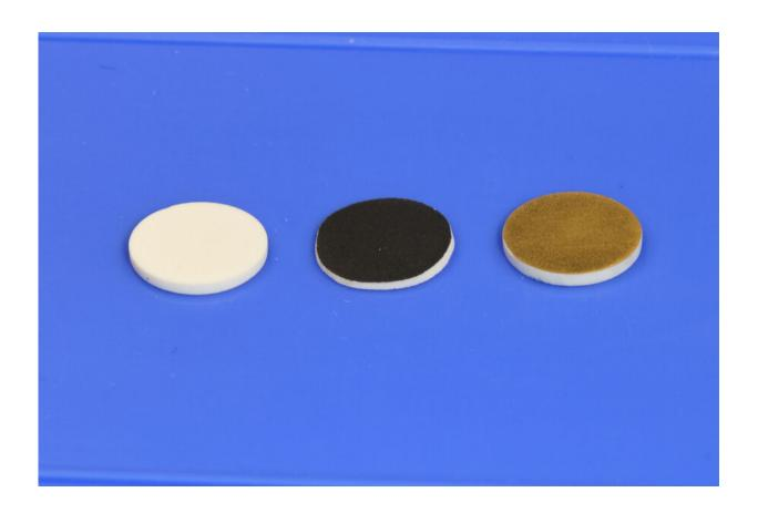
These discs were used for testing the researchers' processing method for solidelectrolyte batteries. On the left, a sample of the solid electrolyte itself, a material known as LLPO. At center, the same material coated with the cathode material used in their tests. At right, the LLPO material with a coating of gold, used to facilitate measuring its electrical properties. Credit: Pjotrs Žguns
