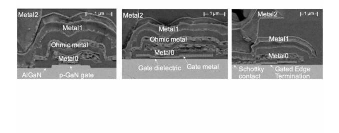
Process cross-sections of the high-voltage components fabricated on 200 mm GaN-on-SOI substrates (a) e-mode pGaN-HEMT (b) d-mode MIS-HEMT, (c) Schottky barrier diode. All devices include metal field plates based on front-end and interconnect metal layers and separated by dielectric layers. Credit: IMEC
