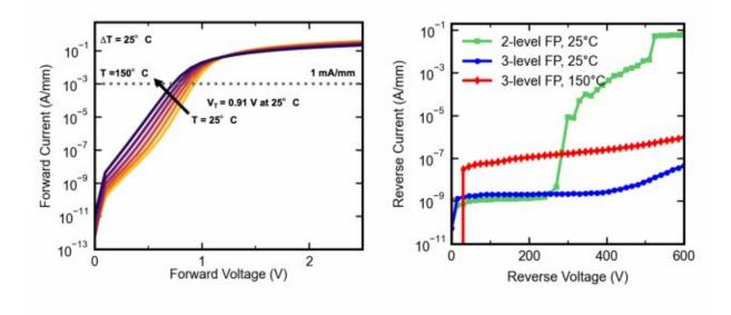
Characteristics of manufactured GET-SBDs showing (left) low turn-on voltage of 0.91V at 25°C in semi-log scale, and (right) low reverse leak currents (2 nA/mm for 25°C) for two different anode field plates configurations evaluated at 25 and 150°C. Credit: IMEC
