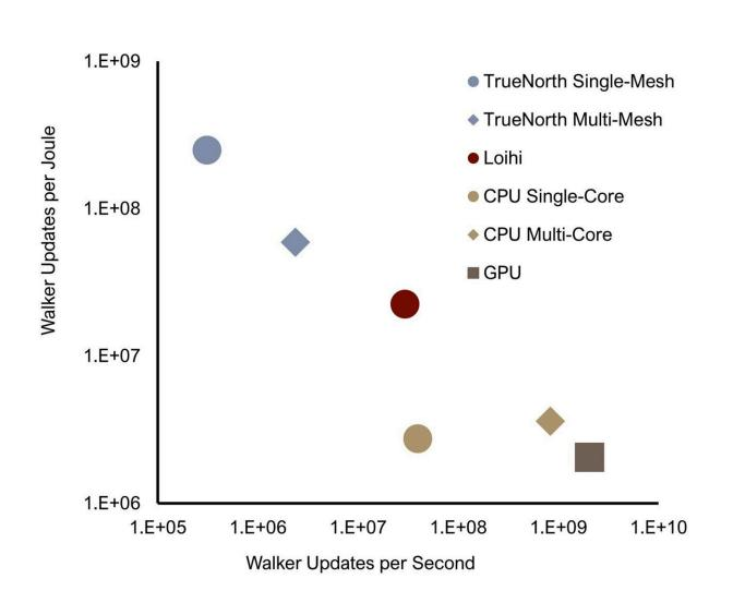
Showing a neuromorphic advantage, both the IBM TrueNorth and Intel Loihi neuromorphic chips observed by Sandia National Laboratories researchers were significantly more energy efficient than conventional computing hardware. The
