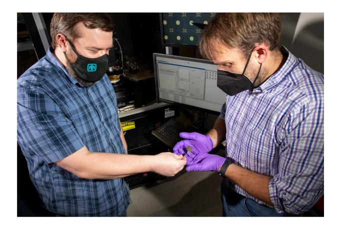
Luke Yates, left, a Sandia National Laboratories electrical engineer, passes Jack Flicker, a grid resiliency expert, a gallium nitride wafer with an array of diodes that can shunt a record-breaking 6,400 volts of electricity within a few billionths of a second. Credit: Rebecca Gustaf
