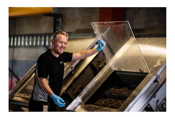
Phosphorous recovery: Bacteria are helping the phosphorous in decontaminated wastewater to be converted into an eco-friendly fertiliser. The product, struvite, has been approved as an organic fertiliser. Credit: HIAS in Hamar
