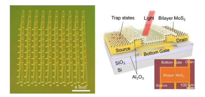
A photograph of the bio-inspired vision sensor array on a diced  $2.5 \times 3.0$  cm<sup>2</sup> chip (left), and schematic structure and optical microscope image of a single vision sensor (right). Credit: Liao et al.
