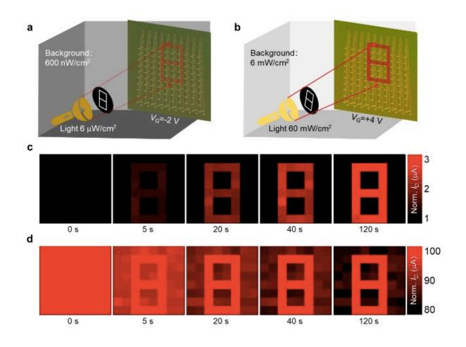
Scotopic and photopic adaptation of the bio-inspired vision sensor array. (a) Schematic illustration of an 8×8 pixel array under a dark background to recognize low-intensity image for scotopic adaptation test. (b) Schematic illustration of an 8×8 pixel array under a bright background to recognize strong light image for photopic adaptation test. The time-course of (c) scotopic and (d) photopic adaptation for the pattern of "8". Credit: Liao et al.
