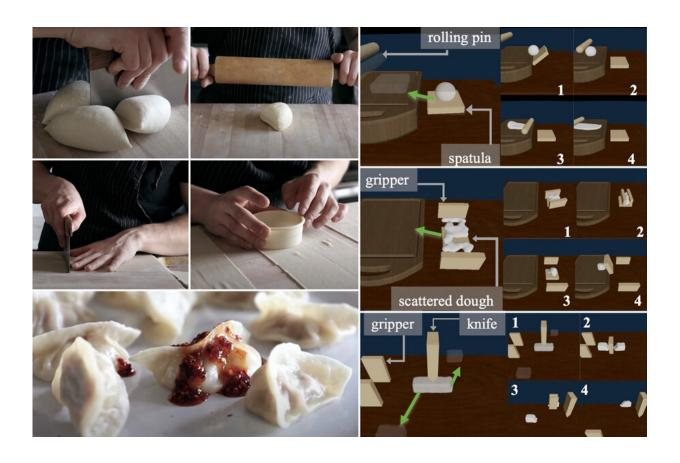
Researchers from MIT and elsewhere have created a framework that could enable a robot to effectively complete complex manipulation tasks with deformable objects, like dough or cloth, that require many tools and take a long time to complete. Credit: Massachusetts Institute of Technology
