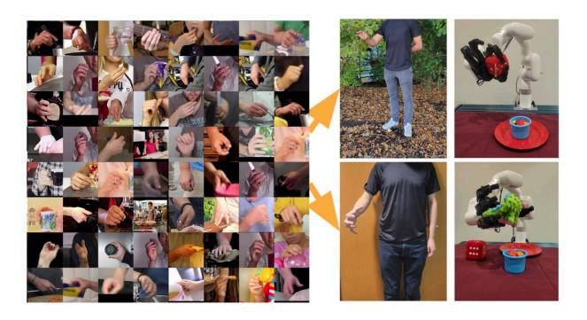
Robotic Telekinesis leverages passive data from the internet to enable real-time teleoperation of a dexterous robotic hand in the wild. Credit: Sivakumar, Shaw & Pathak.
