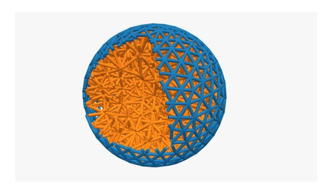
Wrapping an elastic ball (orange) in a layer of tiny robots (blue) allows researchers to program shape and behavior. Credit: Jack Binysh
