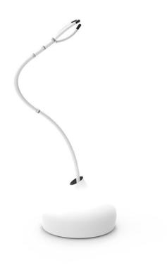
Design study of the appearance of a streamlined robot arm with high potential acceptance for use in close proximity to humans. Credit: L. Boxberger/Fraunhofer IWU
