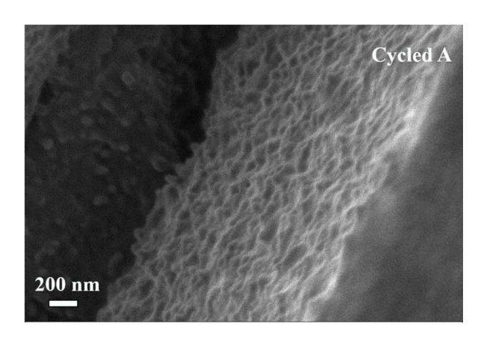
SEM image of the cross-section of the optimal Si film electrode after cycling. Credit: Vesa-Pekka Lehto
