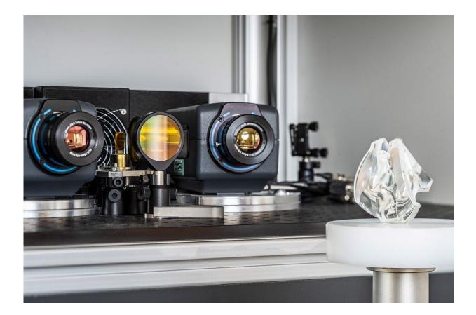
The system works with thermal radiation for the 3D detection of transparent objects. Credit: Fraunhofer-Gesellschaft
