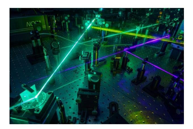
In the femtosecond laser laboratory of Dr. Dennis Friedrich at HZB, the transport properties of semiconductors can be determined using terahertz or microwave spectroscopy. For this purpose, a laser light pulse first excites the charge carriers in the material, which are then irradiated with electromagnetic waves (either THz or Microwave) and absorb some of them. Credit: HZB
