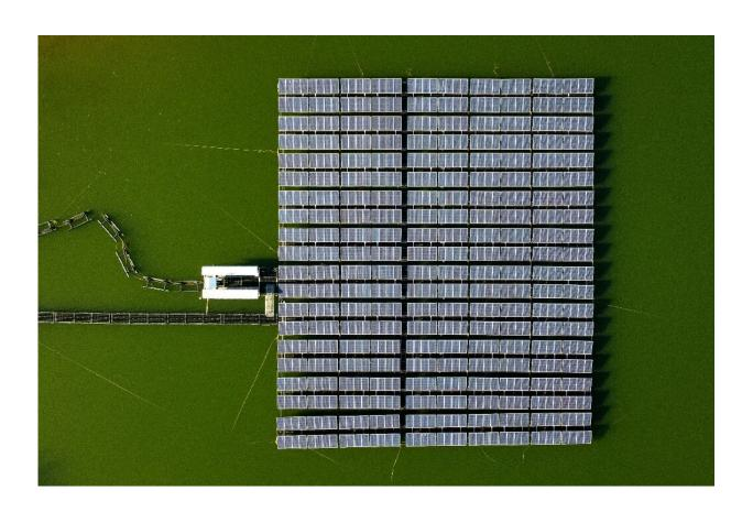
The Sirindhorn Dam covers 720,000 square metres of water surface, is a hybrid system that converts sunlight to electricity by day and generates hydropower at night.
