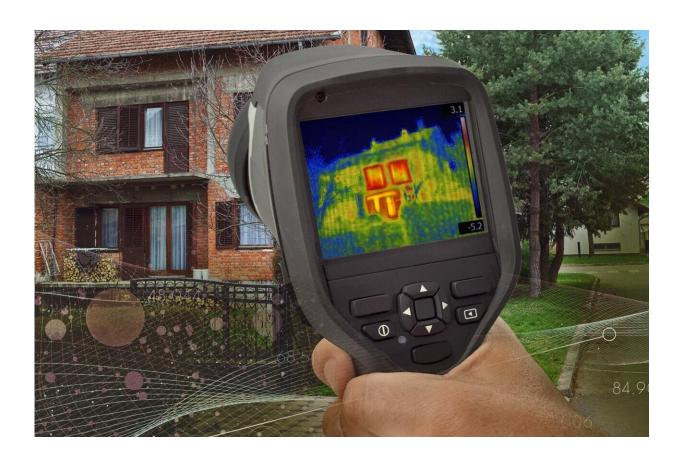
Infrared (IR) imaging technology (shown here) is one of the tools used to measure heat loss through poorly insulated windows. A series of research studies shows that a new generation of triple-pane windows can help improve energy efficiency in homes. Credit: Timothy Holland | Pacific Northwest National Laboratory
