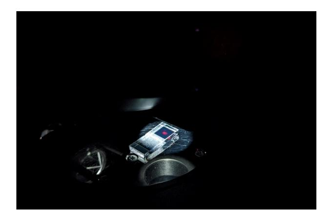
One of the cells fabricated at CSU during characterization. The white beam is the bias light ("the sun"), the red dot is the probe laser. Credit: Onno et al.
