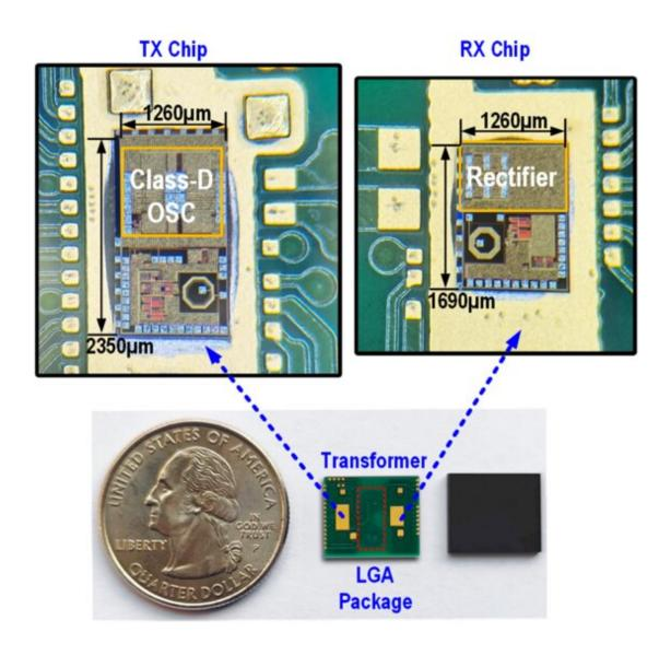
Die micrograph of the RX and the TX chips and a photo of the converter in an LGA package. Credit: Pan Dongfang et al
