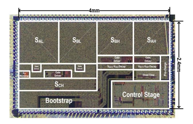
The die micrograph of the DSD converter. Credit: Yuan Jingyi et al
