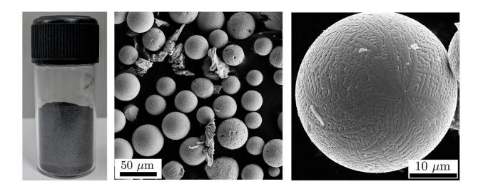
Panel showing metal powders produced using the abrasion-based process. Left: Typical final powder stock after processing. Middle: SEM image showing distribution of powder sizes. Right: Typical single powder particle, approximately 30-50 micrometers in diameter. Credit: Laboratory for Advanced Manufacturing & Finishing Processes (LAMFiP), IISc (mecheng.iisc.ac.in/lamfip)
