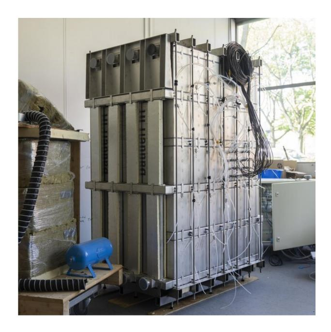
The prototype with the "lockers" that each form a separate module of the thermal battery. Credit: Vincent van den Hoogen
