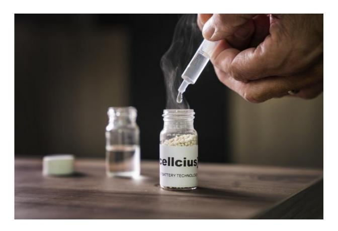
The simple experiment in pictures. A drop of water by the bottle of salt and suddenly a lot of heat is released. Credit: Vincent van den Hoogen
