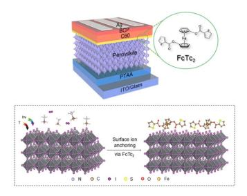
The top picture shows the molecular structure of ferrocene-based metallic compound (FcTc2) and its application in perovskite solar cells. The bottom picture shows the working mechanism of the ferrocene-based metallic compound. Credit: *Science* (2022). DOI: 10.1126/science.abo0039
