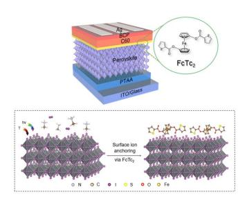
The top picture shows the molecular structure of ferrocene-based metallic compound (FcTc2) and its application in perovskite solar cells. The bottom picture shows the working mechanism of the ferrocene-based metallic compound. Credit: *Science* (2022). DOI: 10.1126/science.abo0039
