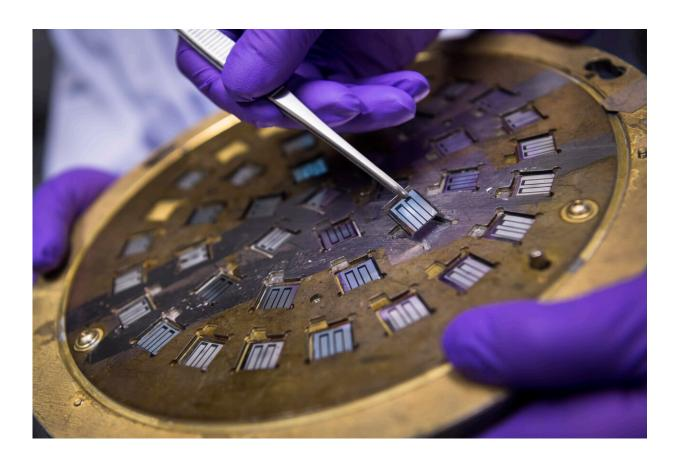
In collaboration with Professor Nicholas Long from Imperial College, Dr Zhu Zonglong's team from CityU ingeniously added ferrocenes to perovskite solar cells as an interface between the light-absorbing layer and the electron transporting layer, achieving a breakthrough. Credit: City University of Hong Kong
