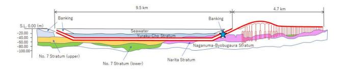
Tokyo Bay tunnel. A cross-section diagram details how the tunnel is situated below Tokyo Bay and the blue star marks the location of the muographic instruments. Credit: Tanaka et al.
