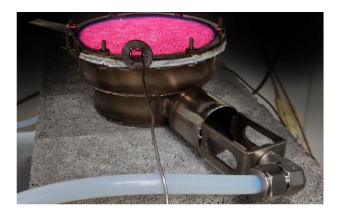
Oak Ridge National Laboratory researchers developed a single burner cooking appliance powered by a blend of 50% hydrogen and natural gas, reducing emissions that contribute to the carbon footprint. Credit: ORNL, U.S. Dept. of Energy
