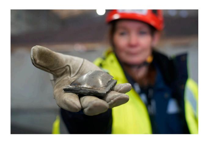
Susanne Rostmark, research leader, LKAB, holds a piece of hot briquetted iron ore made using the HYBRIT process nearby the venture's pilot plant in Lulea, Sweden on Feb. 17, 2022. The steel-making industry is coming under increasing pressure to curb its environmental impact and contribute to the Paris climate accord, which aims to cap global warming at 1.5 degrees Celsius Credit: James Brooks via AP
