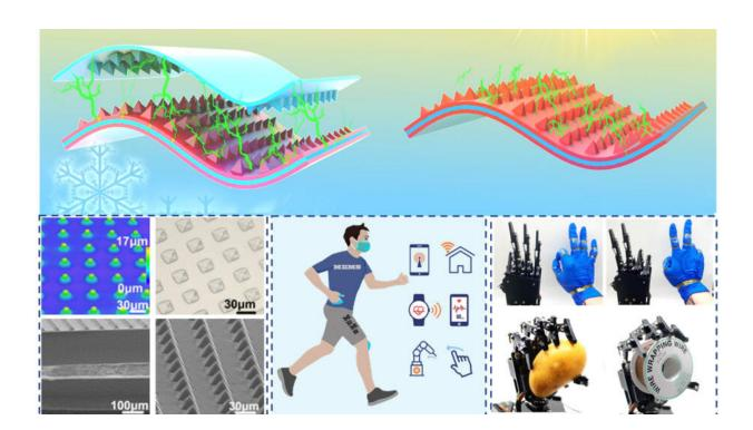
Friction between sophisticated materials with pre-patterned pyramid shapes, used to make the sensor, can generate enough energy to power wearable devices. Credit: Northumbria University
