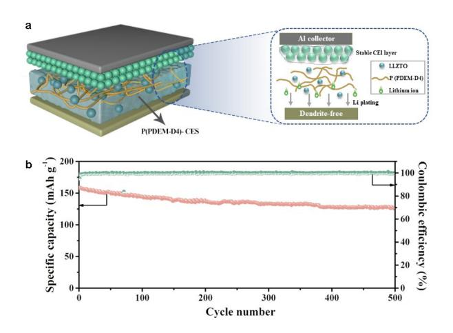
Schematic diagram of CSE design and cycling performance of the as-assembled 4.4 V-class LiCoO2/Li metal battery. Credit: Science China Press
