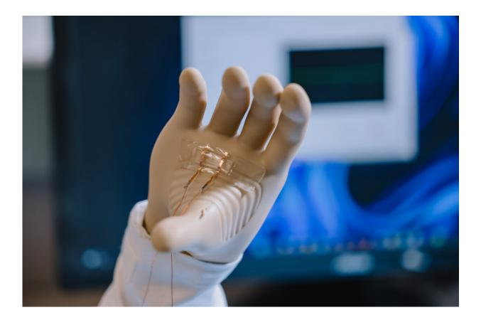
Photo shows the hydrogel sensor attached to a prosthetic arm. When pressure is applied to the sensor, it prompts the arm to move. Credit: Kai Jacobson/UBC Faculty of Applied Science
