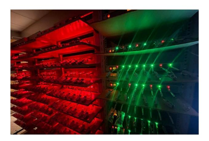
Hundreds of batteries sit on massive racks, blinking red and green, and are tested everyday inside Feng Lin's lab. The green and red lights mean the testing channels are working. Credit: Feng Lin.
