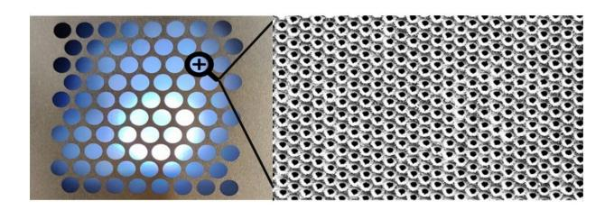
In the microplastic filter, the films with the microholes are fixed on a coarser grid so that they do not tear under the water pressure. Credit: Fraunhofer ILT, Aachen
