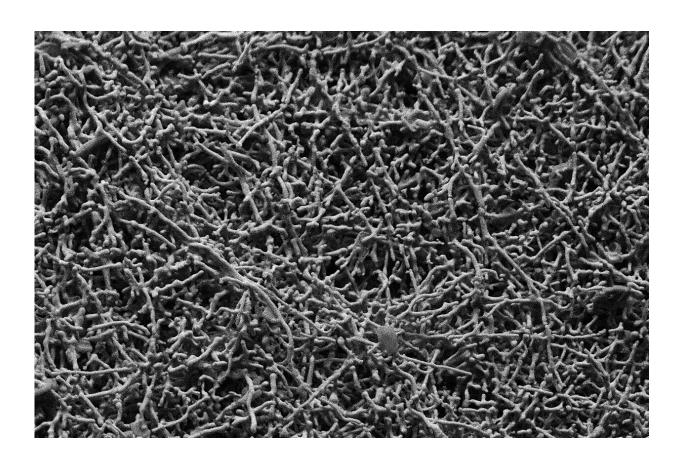
Nanowires made out of a lithium-oxide garnet ceramic filler known as LLZO as seen under a scanning electron microscope. Credit: Rettenwander et al. (2021)
