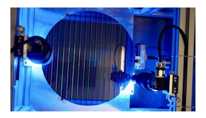
The device uses two cameras to capture the wafer's edge. Credit: University of Colorado at Boulder
