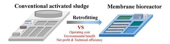
Techno-economic performance comparision before and after the retrofitting of wastewater treatment plants from the conventional activated sludge process to the membrane bioreactor process. Credit: Higher Education Press Limited Company
