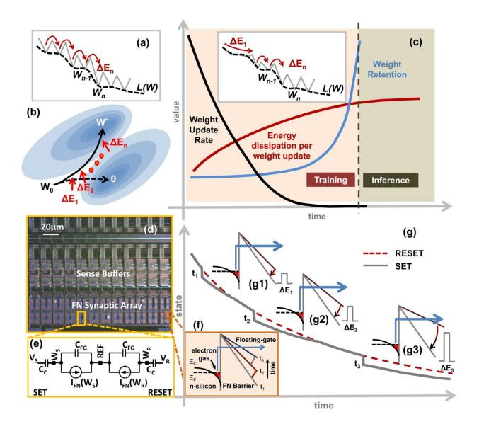
Motivation and principle of operation for the proposed synaptic memory device. (a) Conventional non-volatile analog memory where transition between analog
