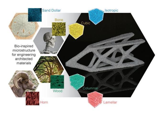
Designed to mimic bone, wood and other natural materials, the porous objects are lighter than traditional products and can be strategically inserted into structures to provide higher stiffness in areas with high demand. Credit: Paulino et al
