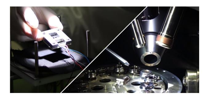
The left-hand side shows a contacted tandem solar cell in the solar simulator at the University of Wuppertal, the right-hand side the apparatus for measuring the energy levels using photoelectron spectroscopy at the University of Cologne. Credit: left: Cedric Kreusel, Wuppertal, right: Selina Olthof, Cologne
