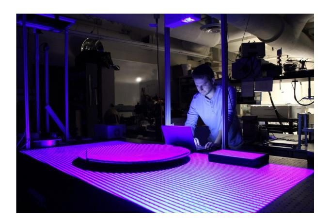
Doctoral student Joel Berkson uses a combination of laser projectors and cameras to create a 3D computer model of radio antenna surfaces. Credit: Paul Tumarkin/Tech Launch Arizona
