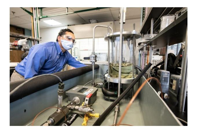
NREL researcher Sreekant Narumanchi uses a liquid cooling loop to characterize reliability of the NREL-designed dielectric fluid jet impingement cooling approach. Credit: Dennis Schroeder, NREL
