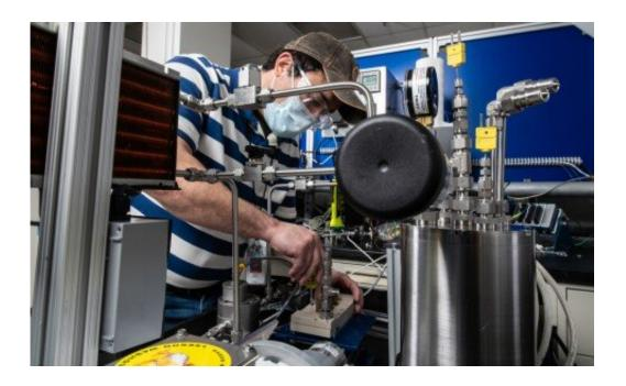
NREL researcher Gilbert Moreno preparing experiments on the dielectric fluid loop to evaluate heat transfer of electrical system component. Credit: Dennis Schroeder, NREL
