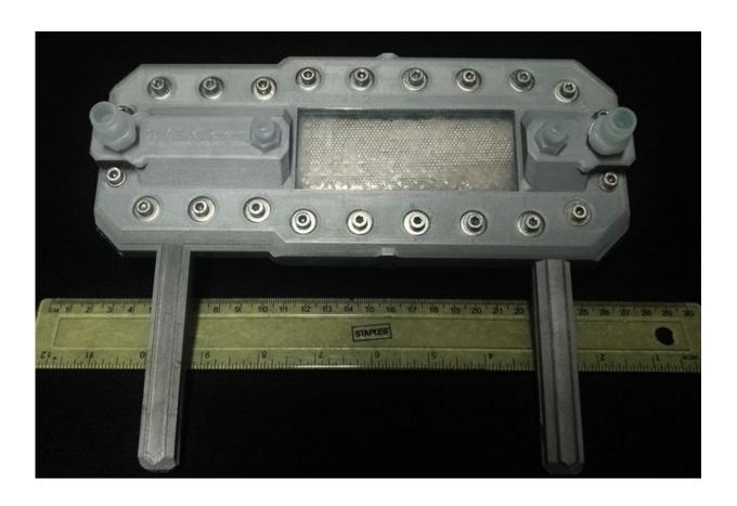
An example of an electrolyzer Weusten managed to build using a 3D-printer. Credit: Eindhoven University of Technology
