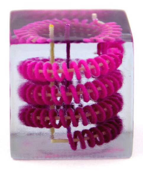
A spiraling pattern created by mixing solid and liquid 3D-printed materials. Credit: Hayes et al. 2022, *Advanced Materials*
