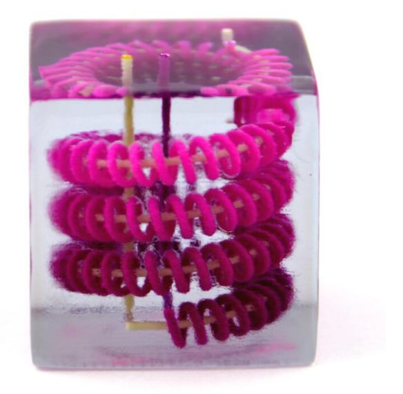
A spiraling pattern created by mixing solid and liquid 3D-printed materials. Credit: Hayes et al. 2022, *Advanced Materials*
