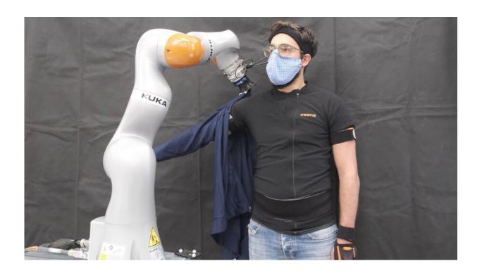
The robot seen here can't see the human arm during the entire dressing process, yet it manages to successfully get a jacket sleeve pulled onto the arm. Credit: MIT CSAIL
