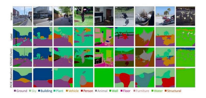
Unsupervised semantic segmentation predictions on the "CocoStuff 27" segmentation challenge. STEGO does not use labels to discover and segment consistent objects. Unlike prior algorithms, STEGO's predictions are consistent, detailed, and do not omit key objects. Credit: MIT CSAIL
